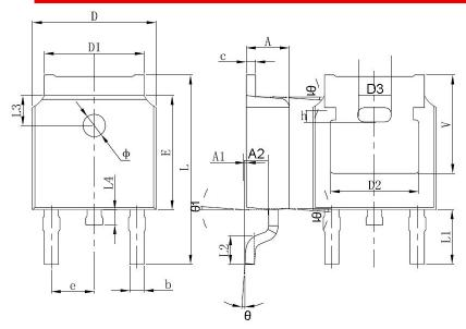
The outline from different package houses may have slight differences. So the outline above is just schematic. The dimensions are controlled per specifications.
